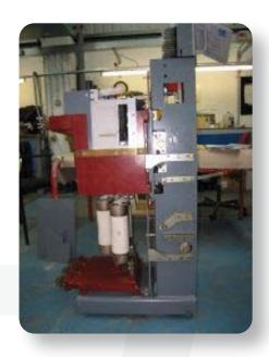
Our S14 contactor range has been designed for total reliability. It utilises a new vacuum contactor which is designed to achieve trouble free performance over many thousands of maintenance free operations.
