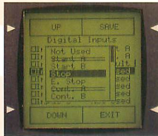
Selecting Digital Inputs. If a digital input has already been set it is struck off the drop-down list. EG Start A
