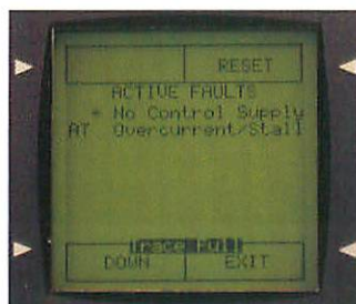
Active Faults page. A&T denotes Alarm and Trip as set earlier.
