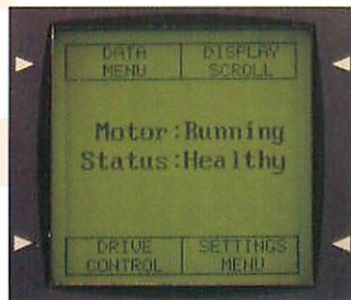
Display Scroll showing drive status information.
